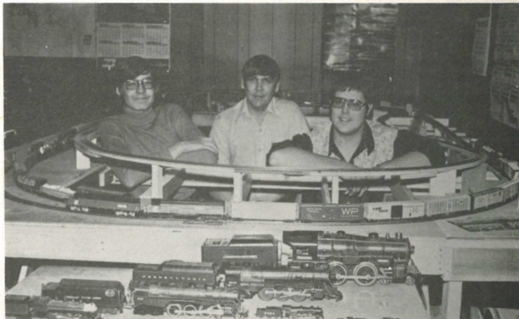
The model railroad engines in the foreground include from the back, a standard gauge, an O gauge, an S gauge, an H0 gauge. The small ones in the front are the longest and shortest N scale models, and the Z scale which is about one inch in length is farthest right in front.
